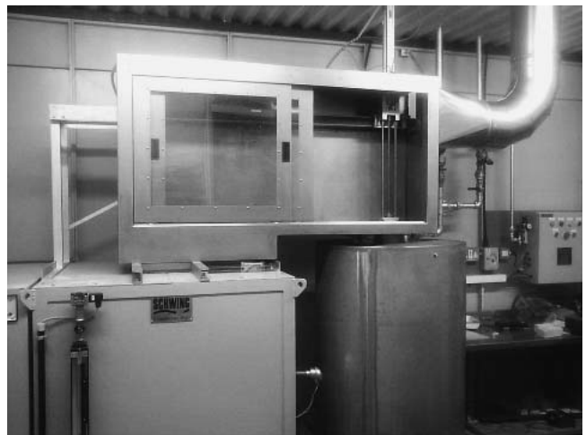
Fig. 12 Fluidized bed thermal shock rig in PST Weston-super-Mare, UK
