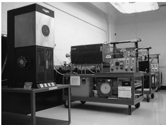
Fig. 5 Bottom-loading furnace and horizontal tube furnaces for cyclic FCT testing of TBC/bondcoat systems
